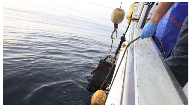
Figure 2. Deployment of the AUSOMS-mini Plus passive acoustic recorder in Ōhata, Aomori Prefecture, Japan. The recorder was lowered from a research vessel and installed at a depth of 29.2 meters using a mooring configuration.
