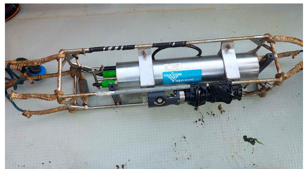
Figure 3. Close-up view of the AUSOMS-mini Plus recorder before deployment. The unit is enclosed in a protective frame and equipped for subsurface mooring.
