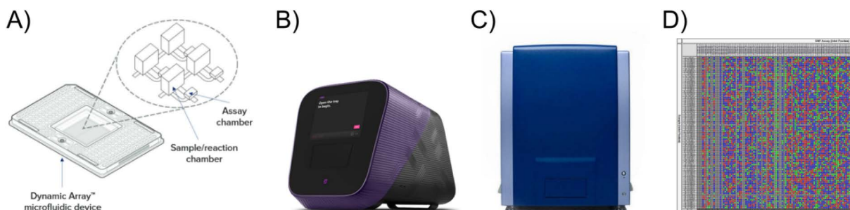
Figure 1. Fluidigm system consisting of (A) the IFC available in different sizes 24×96, 48×48 and 96×96, (B) JUNO to conduct PCRs and (C) EP1 to visualize results. Example of a result output is shown in (D). Each column is a sample while each row is a SNP. Red dots represent a homozygous call for allele (X/X), green dots represent a homozygous call for allele (Y/Y), blue dots represent a heterozygous call (X/Y), and grey dots indicate unsuccessful amplification. Figures (A), (B) and (C) are from Standard BioTools (2024).
