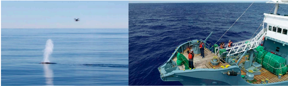
Figure 1. A drone Phantom Pro 4 flying over an Antarctic blue whale during the 2020/2021 JASS-A survey (left). Scene of retrieving the drone Inspire 2 at the bow deck of the research vessel Yushin-Maru No.2 during the 2021/2022 JASS-A survey (right). When retrieving, the drone is caught by hand. For safety, the person catching the drone uses a full-face helmet and cut-resistant gloves.
