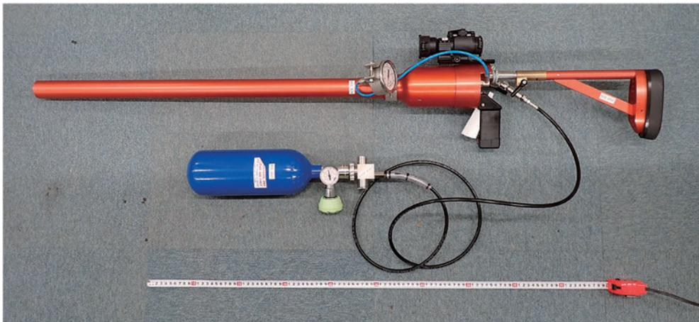
Figure 4. The Air Rocket Transmitting System (LK-ARTS) launching system.
