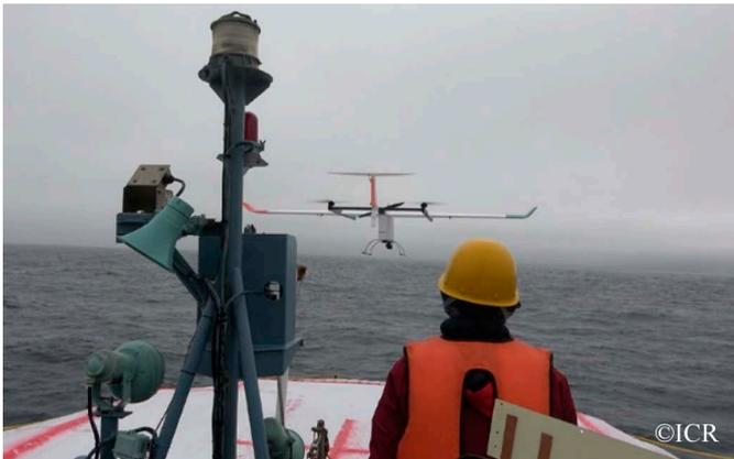
Photo 9. VTOL-UAV ASUKA taking off from onboard.
