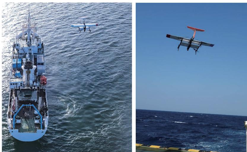
Figure 3. VTOL-ASUKA undertaking vertical take-off from the research vessel (left) and launch landing on the vessel in strong winds (right) during a survey in Mikawa Bay on 29 March 2021.
