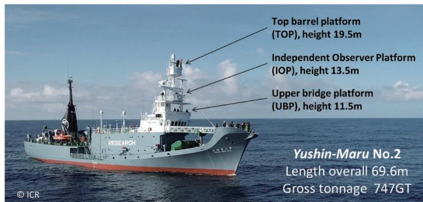
Figure 3. The dedicated sighting vessel *Yushin-Maru* No. 2 and its equipped three platforms.
