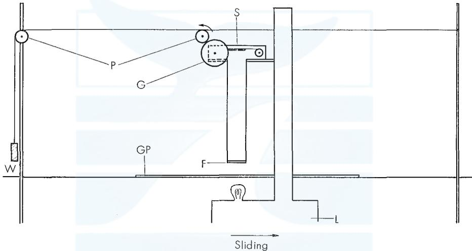
Fig. 4. Diagram indicating the mechanism of photographic apparatus recording the baleen strip. F: filter, L: lathe, G: gear, GP: glass plate, S: slit, P: pulley, W: weight.
