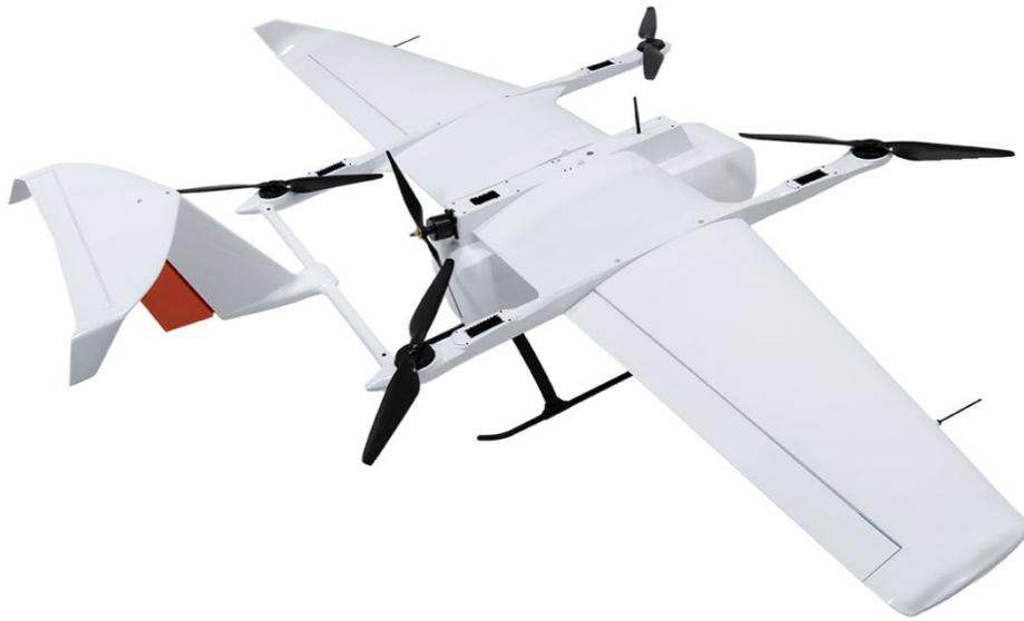
Photo 1: Experimental flight aircraft equipped with hydrogen fuel supply system
