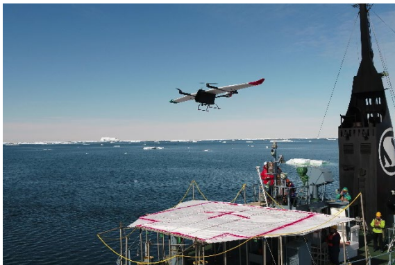
VTOL-UAV ASUKA takes off from the vessel
