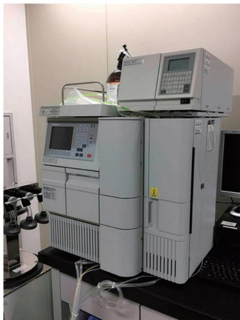
Figure 5. HPCL system (Alliance® HPLC systems e2696, Waters) used for fluorescence detection.
